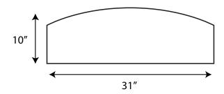
Build Header File as a Complete Rectangle Keeping in mind Arc Guidelines Size should be 31" x 10" plus bleed
